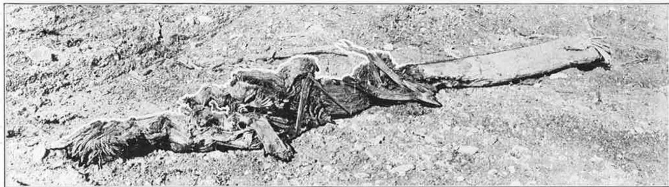
FIG. 375—RESULT OF AN UNSUCCESSFUL ATTEMPT TO DRIVE AN OAK PILE THROUGH COMPACT GRAVEL AT BLACK STREET BRIDGE.
