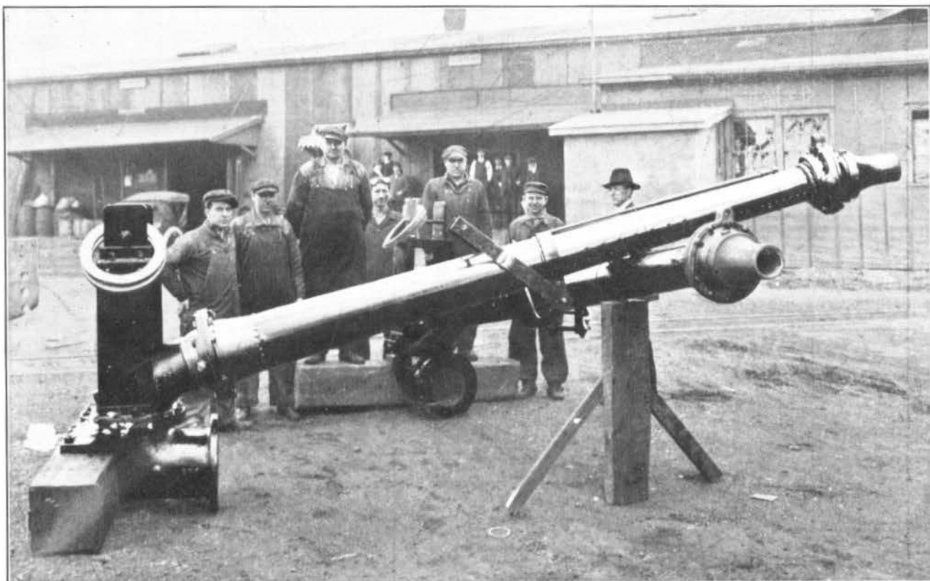
FIG. 111—5-INCH HYDRAULIC "GIANT" FOR LOCKINGTON, MARCH 26, 1920. SEE PAGE 136
