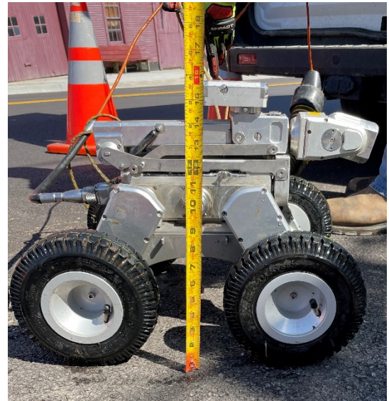
Figure 7: CCTV wheeled camera
