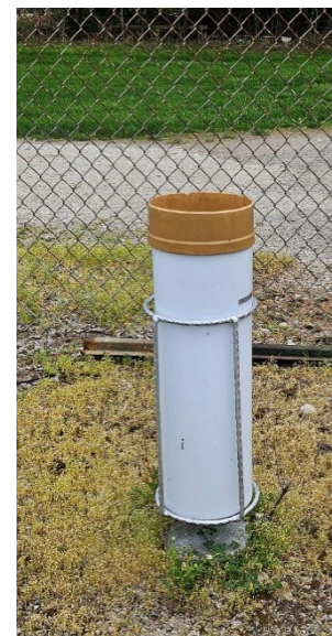
Figure 4 - A National Weather Service standard rain gage.
